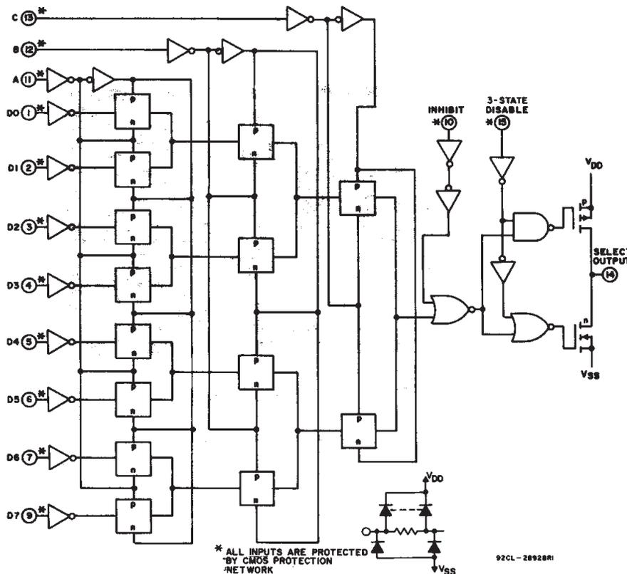
Fig. 1 - Logic diagram.
